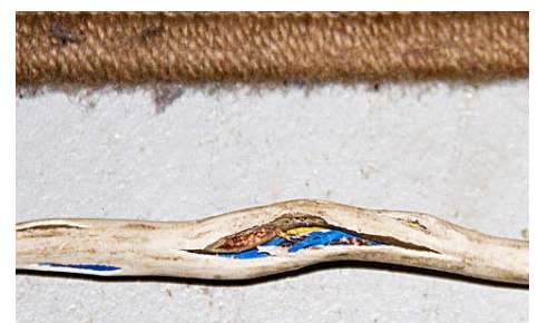
Frayed cords can cause electrical shock or could start a fire.
